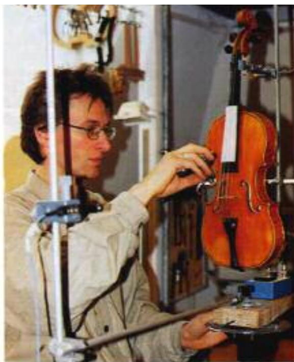
Below Schleske measures the sound radiation of an instrument
