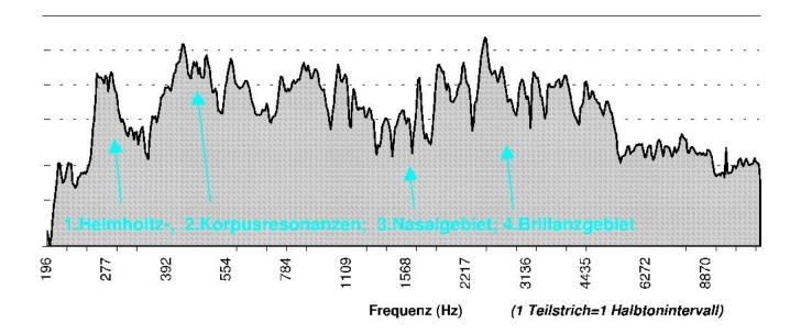
Fig.: Sound energy radiated in all spatial directions by a Guarneri del Gesu violin as a function of frequency. The typical resonance regions are clearly recognizable.
