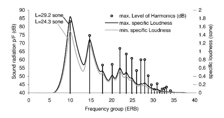
Fig. 1: Excitation pattern of the inner ear when listening to a bowed note played by a violin. Gray curve: Specific loudness due to the minimum harmonic levels within the vibrato shift. Black curve: Specific loudness due to the maximum harmonic levels.
