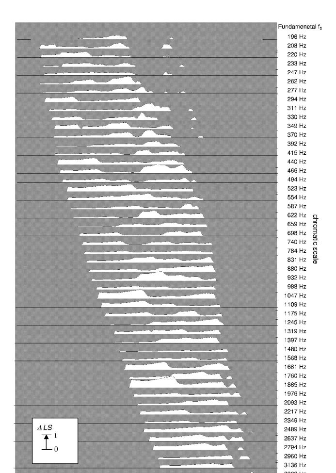
Fig. 2: Depiction of the vibrato sensitivity (and thus the modulability and flexibility of sound) of a violin by Guarneri del Gesu. Vertical axis: Chromatic scale (frequencies of the fundamental pitches). Horizontal axis: "Frequency axis of the inner ear"
