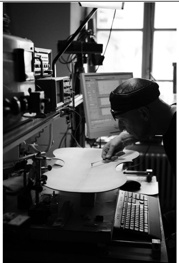
Fig. 1: Modal analysis of a cello top in progress. The coordinate measuring table equipped with linear ball bearings and displacement transducers is used to determine the exact measuring points.
