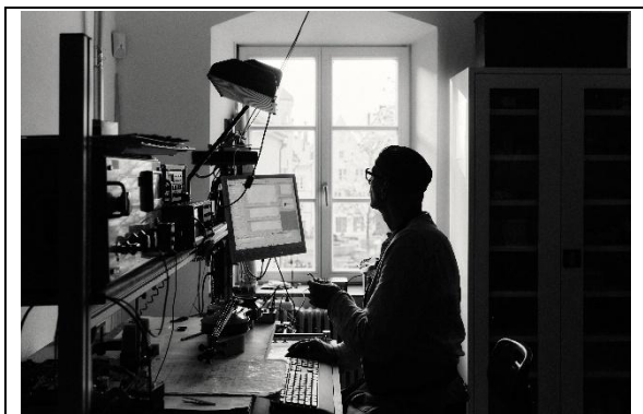
Fig. 3: View of the measuring station for modal analysis of string instruments in our workshop.
