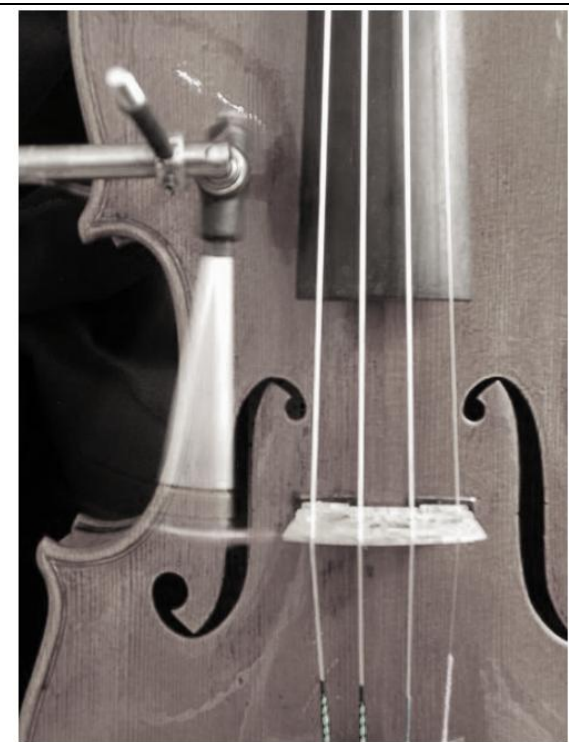
Fig. 5: Excitation mimicry: tripod with ball-bearing impulse hammer pedal.
